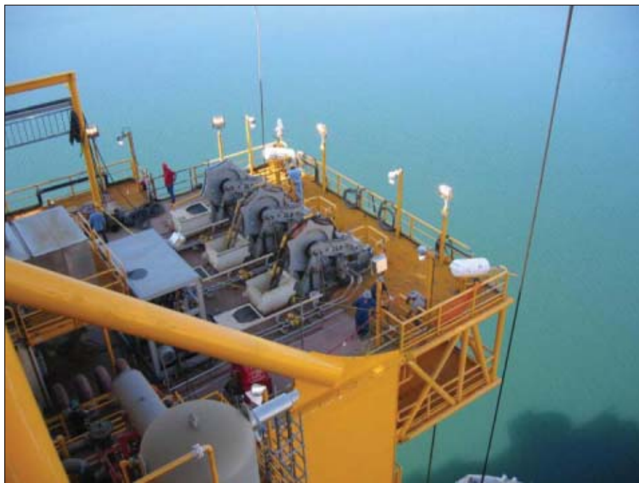
Aker Solutions RamWinches work aboard the Independence Hub in the Gulf of Mexico.
