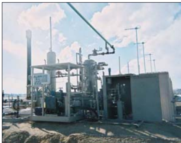
This VRU, integrated with a three-phase separator, was problem prone during several months of testing (Fig. 6).
